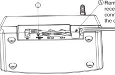
A Remark: Put all the cables inside recess A after all the cables are connected properly for protecting the connection.
